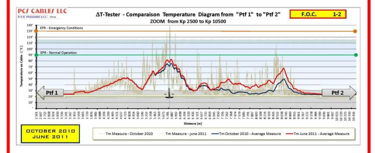
The  $\Delta T$  increase warns about the insulation that is less capable to dissipate conductor heat due to intrinsic causes like a reduced thickness due to extreme ageing or external causes like an anchor damage.
