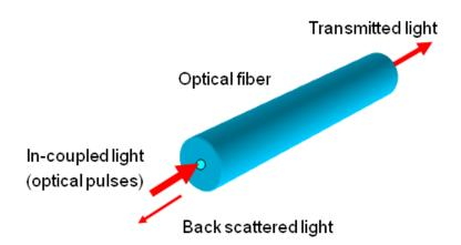
The process of monitoring a composite cable takes advantage of the fact that the optical fibre is in close contact with the cores thus the temperature monitoring is much easier as external factors have less impact on readings. According to the engineering cable data provided by Customers and the actual value related to the cable in service, the operating temperature can be assumed, following the definitions provided in IEC 287 standard.
