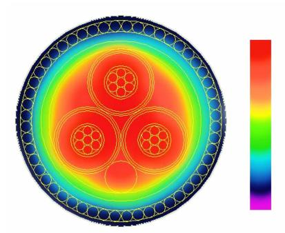
Considering the heat developed by each of the three cores wrapped with optical element and enclosed within binder or inner sheath, cable temperature is slightly higher than working conductor temperature.
